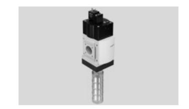
Electro-pneumatic soft-start and quick exhaust valve for gradual pressurisation and quick exhausting of system components (single channel). The main flow control valve in the end cap permits a gradual build-up of output pressure p2. Once the output pressure p2 has reached the set pressure switchover point (switching pressure), the valve opens and the full operating pressure p1 is present at the output.
